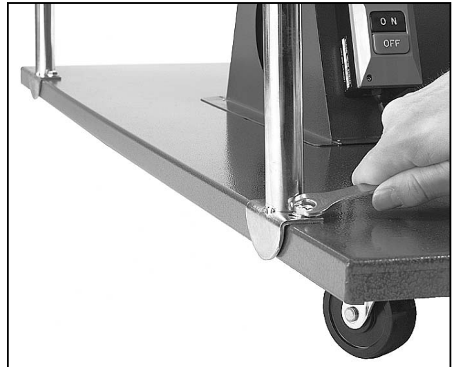
Figure 6. Mounting brackets to base.
